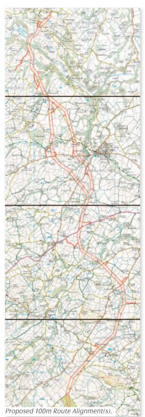
The Project consists of 17km of new 132kV overhead line, together with required accesses, construction laydown areas and other integral works. Rather than specific pole positions, SP Manweb have identified a 100m proposed route alignment within which the overhead line would be sited. This alignment was developed within the broad route corridor (the selection of which was informed by Stage 1 consultation) and itself informed by the feedback received during Stage 2 consultation.
